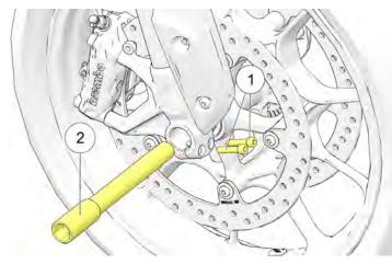
4. Support wheel and remove axle (2) with 22 mm hex drive. Spacers are loosely retained by the dust seals, but may fall out after wheel has been removed.
