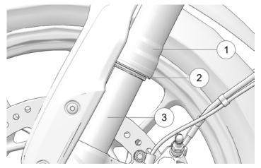
2. Clean the fork tubes to remove bugs, tar or buildup which may cause seal wear or leakage. Inspect the outer surfaces of the inner fork tubes for scratches or damage from foreign objects.
