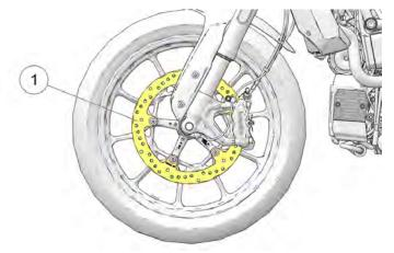
Clean discs if minor squeaks develop due to dirt or dust. Apply brake cleaner to a clean shop towel and wipe the discs. DO NOT allow brake cleaner to contact painted or plastic parts. Read all precautions on the label.
