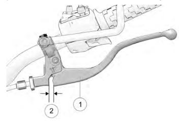
2. Clutch lever freeplay (2) (gap) is the amount of lever movement from the rest position to the point of cable resistance. Measure the gap between the clutch lever and the lever housing. Adjust clutch lever freeplay if necessary.
