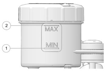
2. View front brake fluid level through the fluid reservoir. The fluid should be clear and between the MIN ① and MAX ② markings. If the fluid level is low, inspect brake pads as outlined on page 126. If pads are not worn beyond the service limit, inspect the brake system for leaks.
