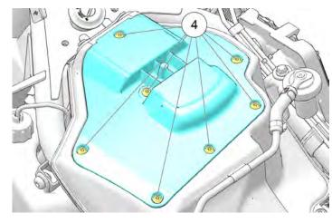
9. Remove the air filter from the airbox.
