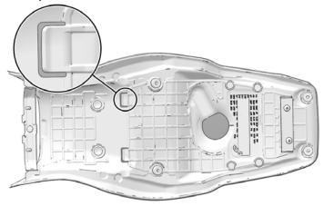
2. Slide the tabs shown above beneath the support bracket and into the front mounting bracket.
