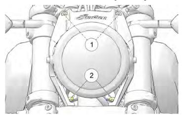
2. Remove and retain two nuts (2) from bottom of headlight bracket.
