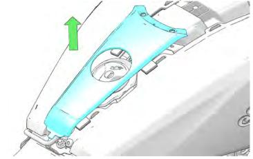
4. Remove the gas cap and relocate to clean, safe location.
