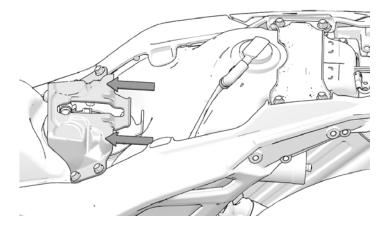
3. Secure the rear of the seat with the two fastener screws.
