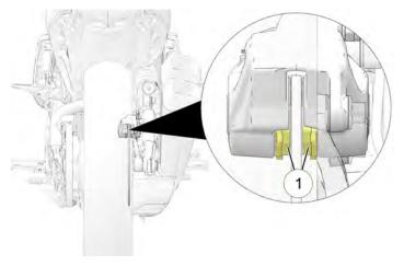
3. Wear indicator grooves should be visible on both inboard and outboard brake pads.
