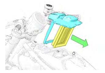
10. Inspect filter element and replace if dirty, wet, or oil fouled.
