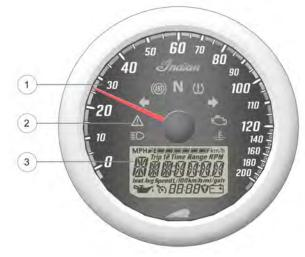
The instrument cluster includes the speedometer, indicator lamps and multi-function display (MFD).
